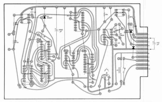
fig. 2. Printed-circuit layout for the RTTY line-end indicator. The unused contacts at R1, R2 and C2 are used, as required, for frequency adjustment. The connection from the collector of the transistor Q1 is chosen for relay or lamp option (see fig. 1). Connect the lamp to pins 2 and 6 of the board. For external power supply, omit the external 100  $\mu$ F capacitor, 120 ohm resistor and 5 volt zener and short pin 1 of the board to pin 2.
